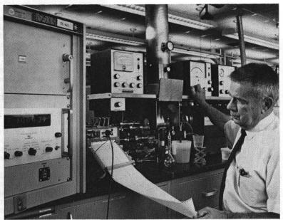
CLEAN AIR TOOLS - Among instruments and technologies in use Ben Seeley (5521) tends the atomic absorption spectrometer, an extremely sensitive device capable of detecting and analyzing minute amounts of metallic elements in an air sample.
